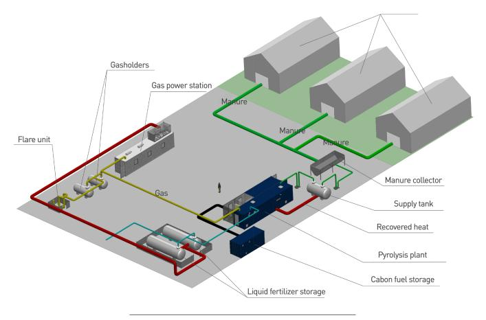
Fig.3. Pyrolysis plant layout diagram.
