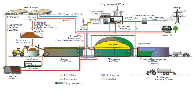
Fig.1. Biogas plant flow chart
