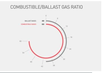
Fig.2. Combustible-to-ballast gas ratio for a biogas plant.
