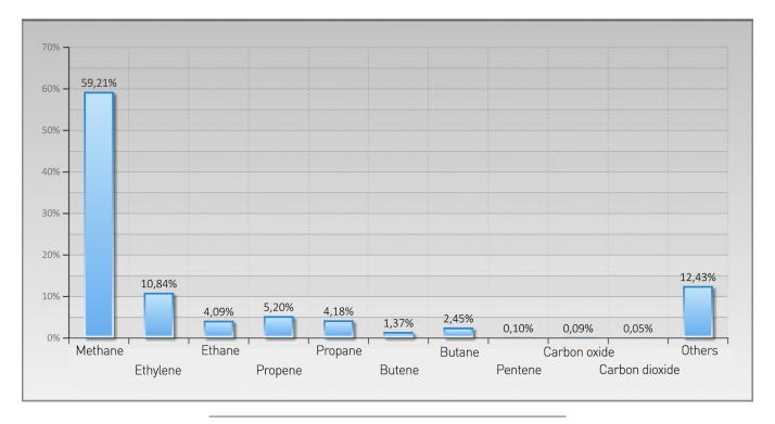
Fig.5. Pyrolysis gas content.
