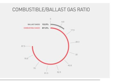
Fig.4. Combustible-to-ballast gas ratio for a pyrolysis plant.
